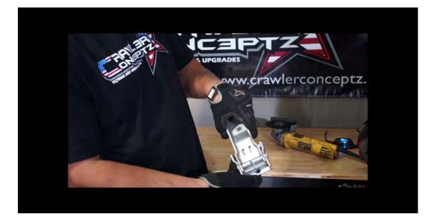
After the pin is cut, pull the pin out and separate the two halves of the hinge. Retain the long half of the hinge that mounts to the tail gate.
