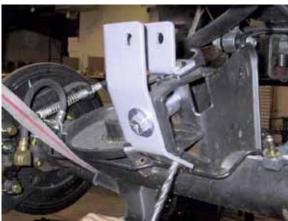
Photo 1 (TJ set up for stock track bar)
