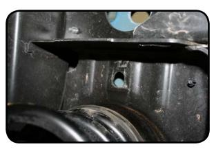
6. Using the supplied hardware, install the coil retainer in between the top to coils. Using a 3/4 socket and wrench torque the bolt to 50 Ft-lbs
